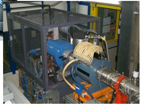
Superconducting ECR source SERSE
